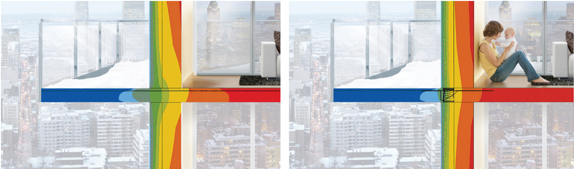
Images showing conduction / heat transfer through balcony with and without thermal break. (Image source: https://www.constructionspecifier.com/ )
